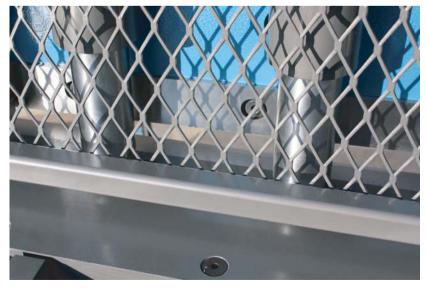
See-thru guard allows operator to see exactly where cut is being made.
